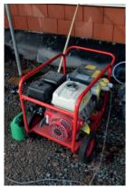
A good supply of power and air pressure is essential, this can be sourced from an on site generator and air compressor, air pressure must be at a minimum of 6 bar.
