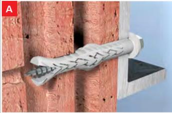
**A** In **hollow building materials** the force is transmitted equally through the two expansion zones. The internal substrate webs are not crushed by the expansion zones and so transmit the force safely.
