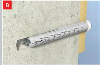
**B** In **solid building materials and aerated concrete** the two expansion zones combine to form one long expansion element, thus providing for a uniform and even distribution of the load into substrate.
